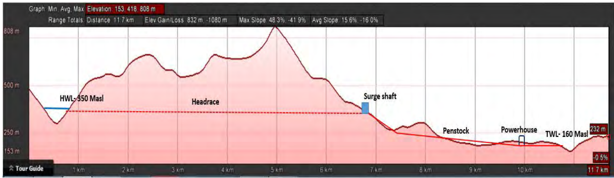
Figure 7.2-10. Profile of NHI Site_D Hydropower Project.
