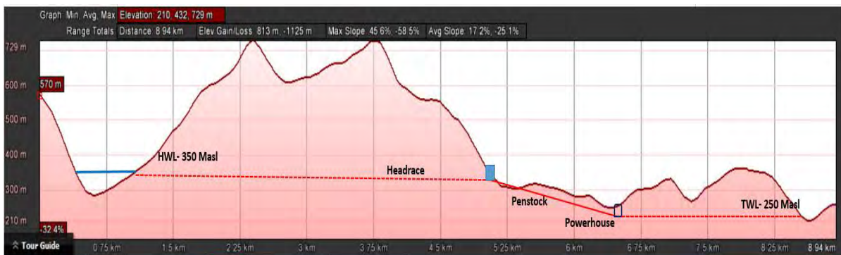
Figure 7.2-8. Profile of NHI Site_C Hydropower Project.
