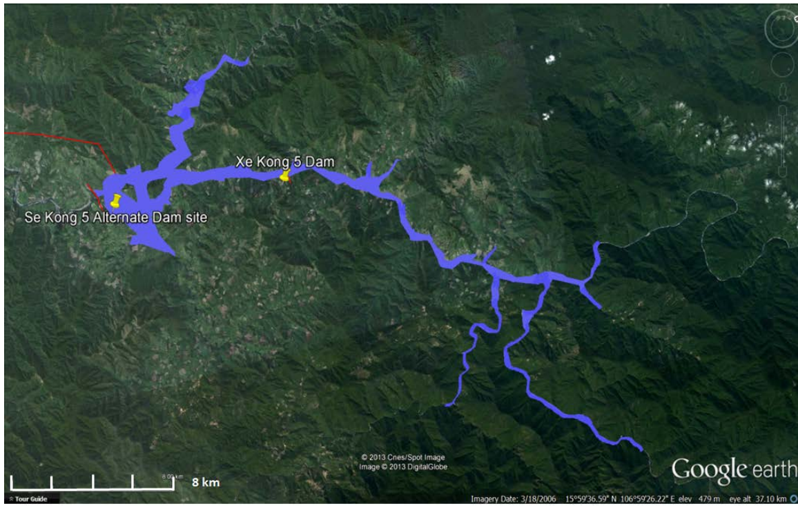
Figure 9.1-12. Reservoir Inundation Area of Xe Kong 5 Alternative-1.
