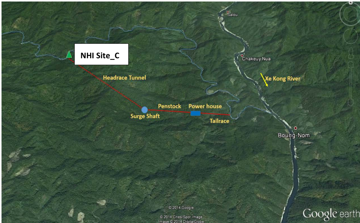
Figure 7.2-7. Layout of NHI Site_C Hydropower Project.
