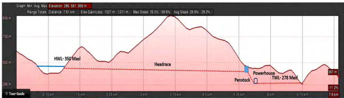
Figure 7.2-2. Profile of Houay Pache Hydropower Project.
