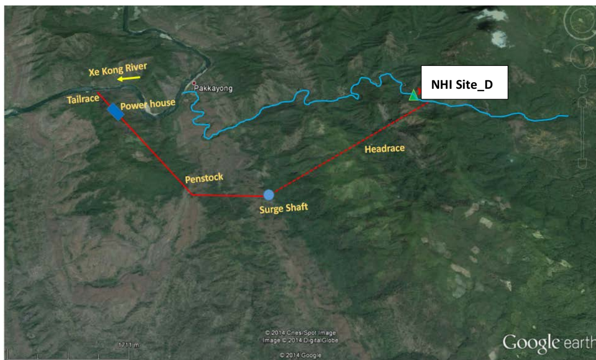
Figure 7.2-9. Layout of NHI Site_D Hydropower Project.
