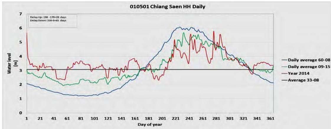
Figure 3.1-2. Water level at Chiang Saen in Thailand south of the Chinese – Thai border. The black line shows long term average. The average from 1960 to 2008 is compared to the average from 2009-2015 where the Chinese dams were filling and commissioned (Green line), and to year 2014 as the most different from average year (red line).
