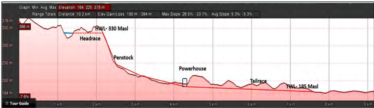
Figure 7.2-6. Profile of Nam Pouang Hydropower Project.
