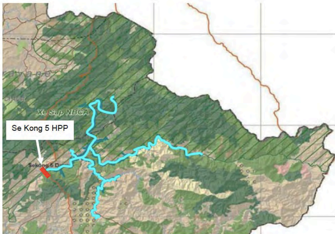
Figure 3.2-22. The upper Xe Kong catchment showing the river that would be inundated (light blue) from the proposed Xe Kong 5 Dam (red) (Norconsult, 2008).
