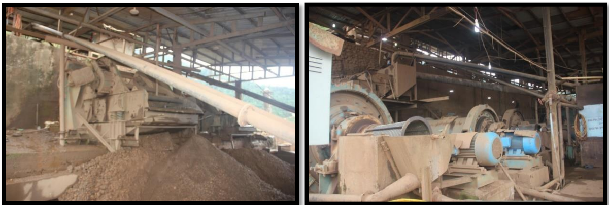
Figure 3.9 Crushing/Secondary breaking: Showing the oversized materials are crushed by ball mill. Oversized blocks are crushed by jaw crusher, sizing by vibrating screen. Then crushed again by ball mill and sized by small trammel to get (-1mm) size.
