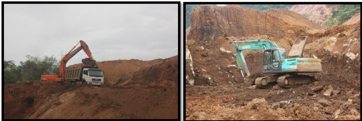
Figure 3.5 Dozing : Showing the alluvial which consists of mixed tin and tungsten and then transported to the dumper. To avoid from mass wasting, ladder shaped benches are made by back-hoe excavator. Bench slope is about 60 degrees and height is 10 meters.
