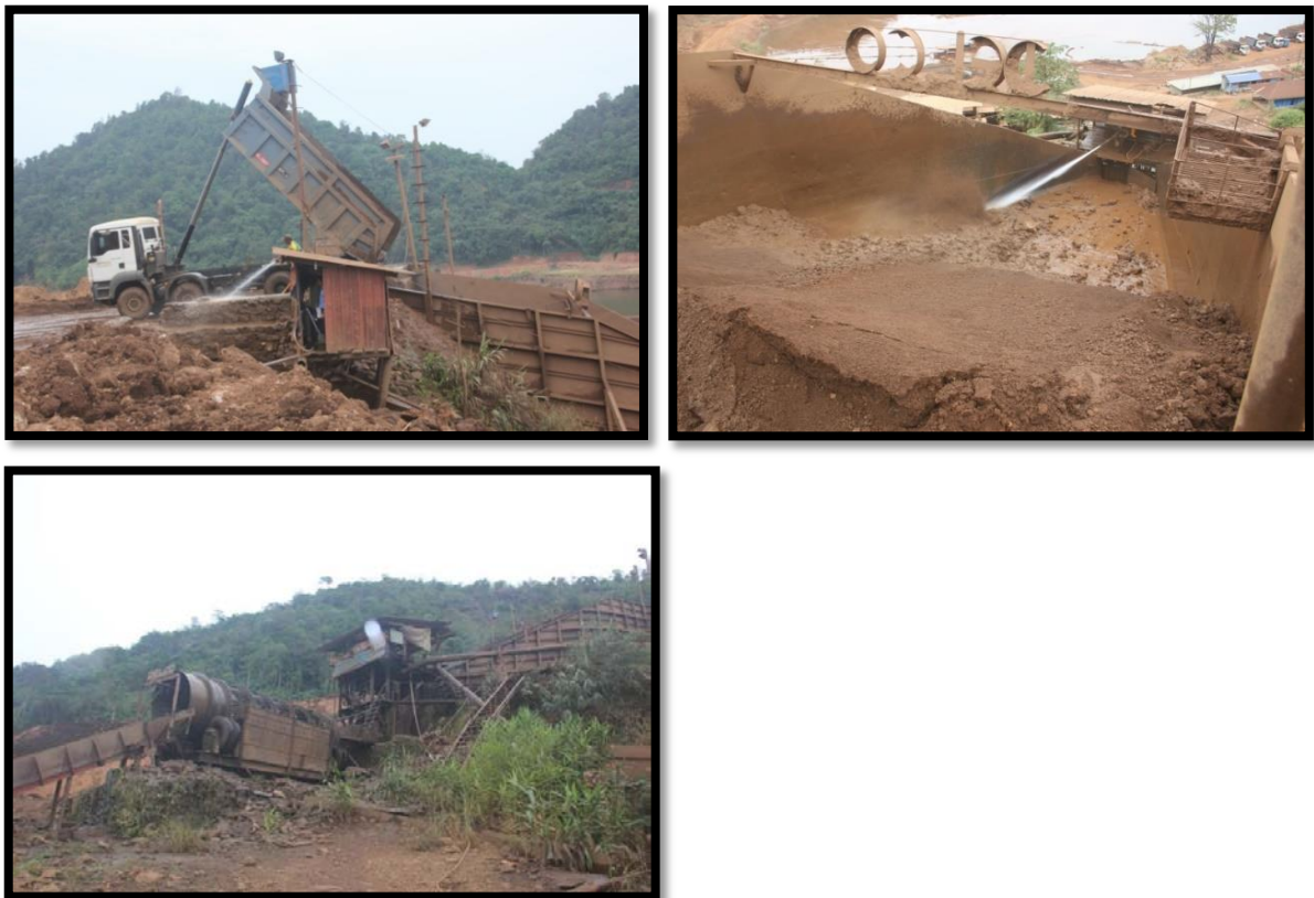
Figure 3.7 Transportation to ore washing bin: Showing the first stage of raw ore materials dumped into washing bin for ore washing by water pump.
