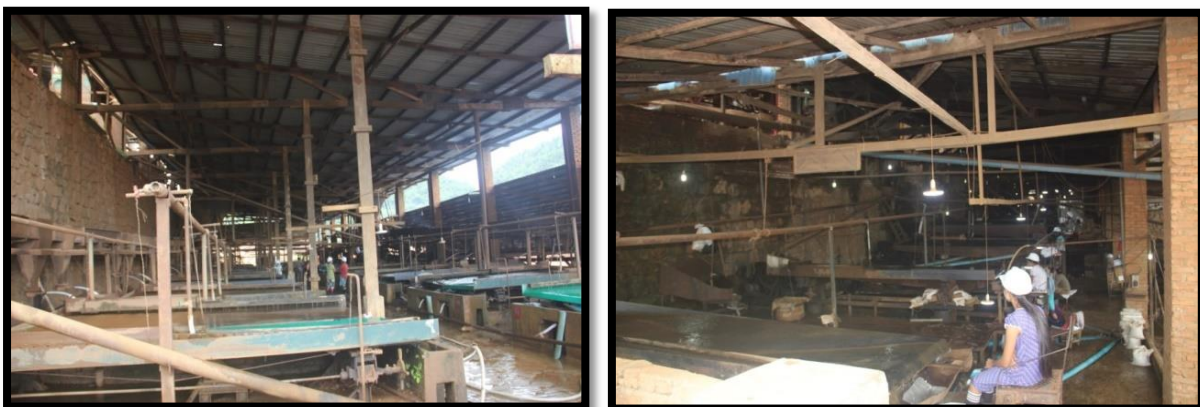
Figure 3.10 Shaking slurry: Showing the two- step shakers for mineral separation. Minus 1 mm sized slurry (mixed soil and mineral) is washed and vibrated step by step by shaking tables to get mineral concentrate. No chemical is used for mineral concentration.
