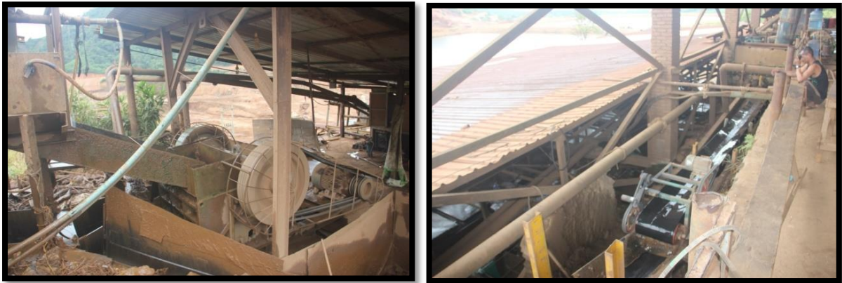
Figure 3.8 Sizing: Showing the washed materials are passed for sizing by trommel. Large trommels at the top level separate the tailings into different sizes which are fed down to the separating tables at the lower levels.
