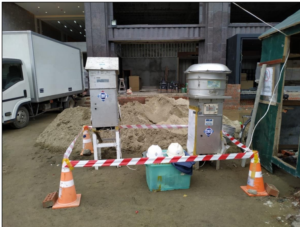
Figure 4-7 TSP and PM 10 Sampling Photo
