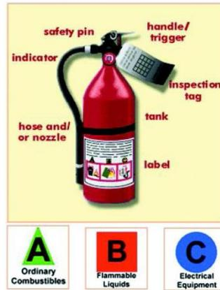
*Components of a fire extinguisher*
