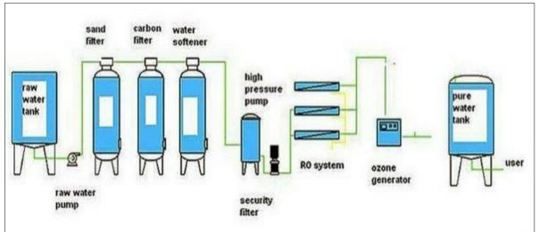
Figure 2.11 Water treatment system for tube well water
