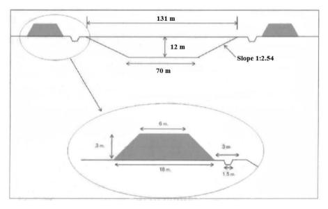
Figure 2.5 Cross section of channel 1
