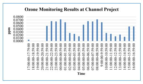
Figure 6.13 Ozone Measurement in Channel Area in March 2019
