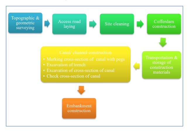
Figure 2.7 Construction Process of the Channel 1
